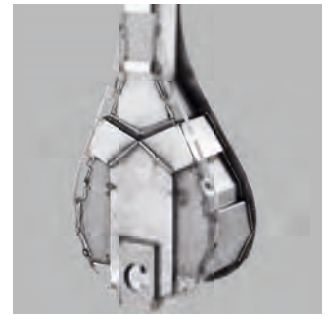
Combustion chamber (back): external air inlet and combustion air preheating.
